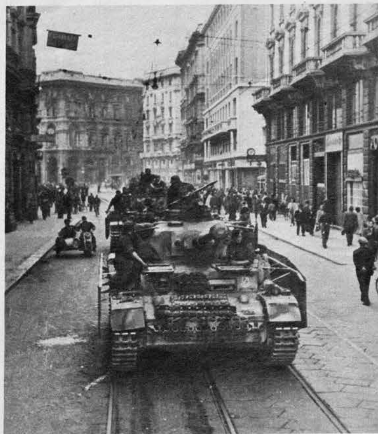
Interesting view of the German Mark IV shows how the armored side skirting, attached to brackets, hangs away from the hull. Notice how extra turret armor stands away from turret, curves toward mantlet.
